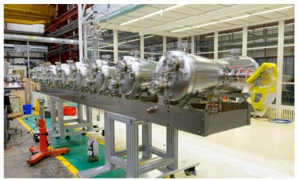
Scientists and engineers at Argonne led the design of these eight accelerator cavities, of a type called half-wave resonators, for the PIP-II accelerator. The Argonne team worked with Fermilab in the design. Credit: Argonne National Laboratory. Fermi National Accelerator Laboratory
