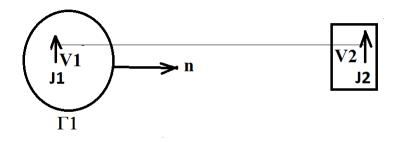
Figure 2: In the volume  $V_1$ , there are only the source  $J_1$ , the sink  $J_2$  is at the outside of the volume  $V_1$ ,  $J_1$  sends the retarded wave  $[E_1, H_1]$ .  $J_2$  sends the advanced wave  $[E_2, H_2]$ .
