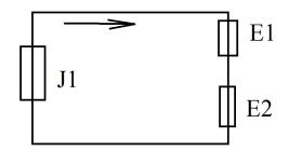
Figure 6: Two loads are connected as series.
