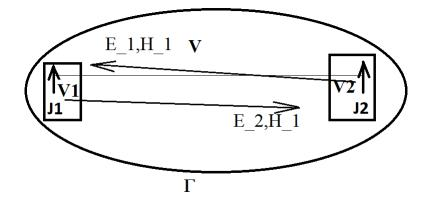
Figure 1: In the volume V, there are source  $J_1$ , sink  $J_2$ ,  $J_1$  sends the retarded wave  $[E_1, H_1]$ .  $J_2$  sends the advanced wave  $[E_2, H_2]$ .
