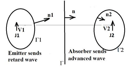
Figure 5: In the volume  $V_1$ , there are only the source  $J_1$ , in the volume  $V_2$  there is the sink  $J_2$ ,  $J_1$  sends the retarded wave  $[E_1, H_1]$ .  $J_2$  sends the advanced wave  $[E_2, H_2]$ .  $\Gamma_1$  is the boundary of volume  $V_1$ .  $\Gamma_2$  is the boundary of volume  $V_2$ .  $\Gamma$  is surface between  $V_1$  and  $V_2$ . The norm vector of the surface are all in the direction from 1 to 2, hence is written as  $\hat{n}_{12}$
