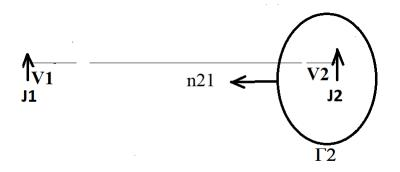
Figure 3: In the volume  $V_2$ , there are only the source  $J_2$ , the source  $J_1$  is at the outside of the volume  $V_2$ ,  $J_1$  sends the retarded wave  $[E_1, H_1]$ .  $J_2$  sends the advanced wave  $[E_2, H_2]$ . The norm vector of the surface is  $\hat{n}_{12}$ .
