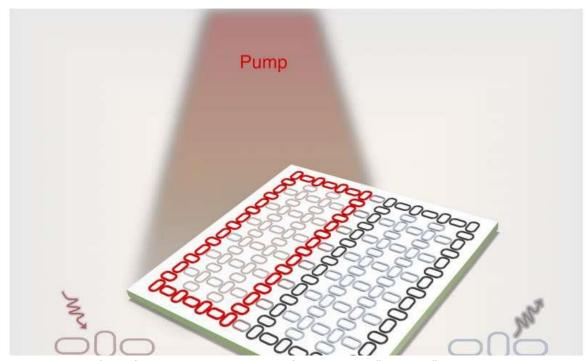
The researchers' chip features a tessellated grid of oval rings. By "pumping" individual rings with an external laser, they are able to dynamically redefine the path photons take. Credit: University of Pennsylvania
