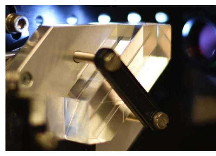
PRISM: microscopy add-on to perform simultaneous 3D imaging of 8 planes. Credit: Vytautas Navikas
