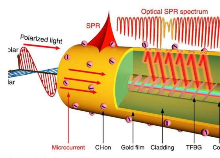
Electrochemical surface-plasmon-resonance sensing principle and experimental demonstration with a gold-coated TFBG optical fiber sensor. Sketch of the configuration of a plasmonic optical fiber sensor for in situ monitoring of ...more
