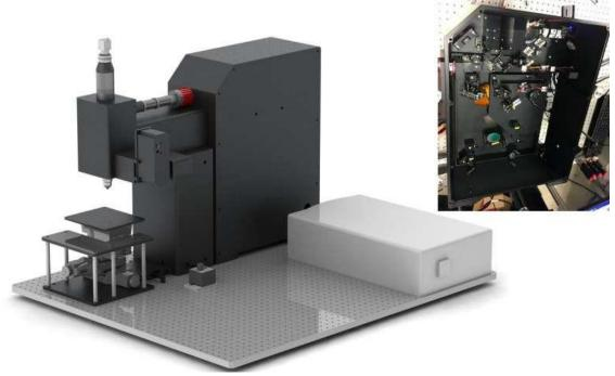
Researchers have developed a system that increases the imaging speed of two-photon microscopy up to three to five times without compromising resolution. On the left is a CAD model of the compact, custom built, two-photon microscopy system. The free-space optics inside are pictured on the right. Credit: The Chinese University of Hong Kong
