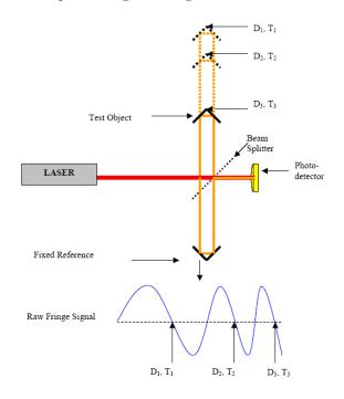
FIG. 3. Direct Measurement of g
