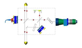
FIG. 2. Beam Path in FG5 interferometer
