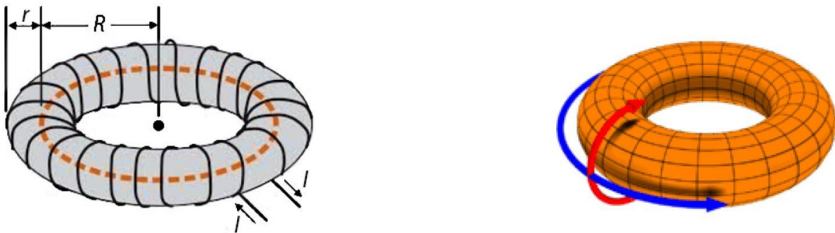
Figure 4: Consa's Helical Electron Model (toroidal versus poloidal currents)
