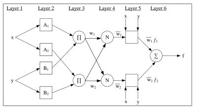
Figure 1. Adaptive network based fuzzy logic inference system (ANFIS)
