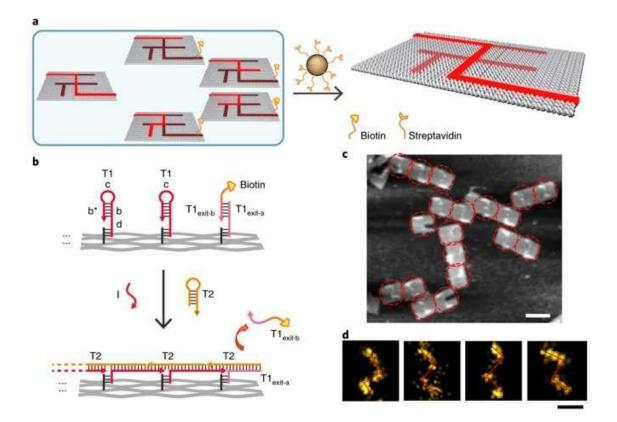
Single-molecule DNA navigators for maze-solving. a) Schematic illustration of magnetic bead-based selection. Exit vertex J is labelled with biotin to enable differentiation between the correct and wrong paths. Only if the PSEC reaches the ...<u>more</u>
