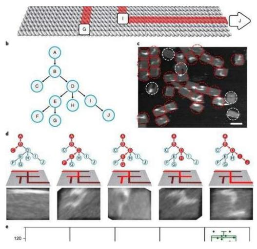
The PSEC-driven graph traversal on a maze. a) A maze design with 10 vertices. Arrows indicate the entrance vertex A and exit vertex J. b) The maze is equivalent to a rooted tree with 10 vertices. The entrance vertex A corresponds to the ...<u>more</u>
