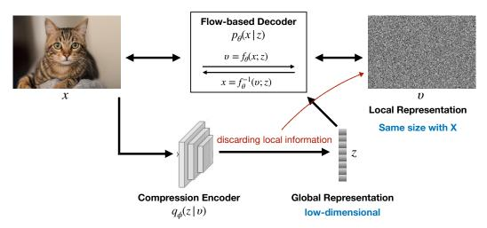
Figure 2: Diagram to illustrate the process of decoupling an image x into the global representation z and local representation v. The key insight is the architecture design of the compression encoder and the invertible decoder.
