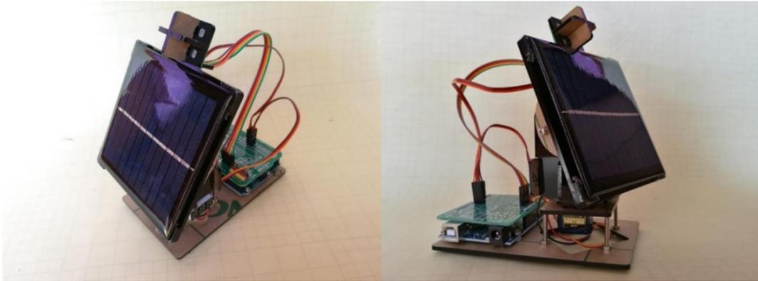
Fig.4.The actual model of the created solar tracking system
