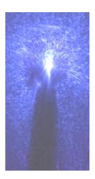
Fig. 17.3. Image of a shadow from a magnetic ball when a blue laser beam passes around the ball from above. The beam is diffracted in the boundary layer of the ball and extends far into its shadow area.
