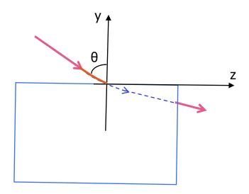
Fig. 15.2. Side view of the plates. The dotted line shows the beam path for the region in which the closer plate blocks our view of the beam.
