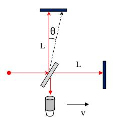
Fig. B1. The Michelson interferometer moves along with the Earth in its motion around the Sun.
