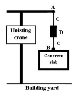
Figure 2. Lifting of the cargo (concrete slab) is the work which is performed by the hoisting crane. c is a steel cable; D is a dynamometer which measures the confining force of the steel cable c.
