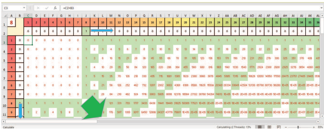
Figure 7 – illustrating how the Sierpiński pattern grows in diagonally as the 'inputs' are turned on sequentially by manually increasing cell A1..
