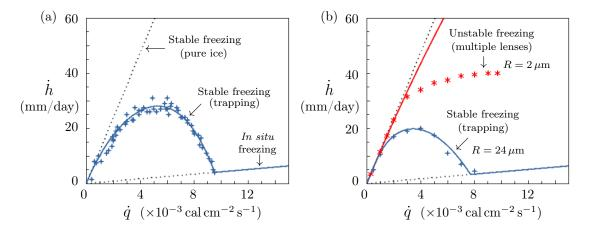
Figure 3: Total frost heave rate  $\dot{h}$  versus the heat extraction rate  $\dot{q}$ . The data in (a) are from Horiguchi [4] using  $R=20\,\mu\mathrm{m}$  zeolite particles, while the data in (b) are from [4] using carborundum particles with  $R=24\mu\mathrm{m}$  (crosses) and  $R=2\mu\mathrm{m}$  (stars). The curves are from equation (26).
