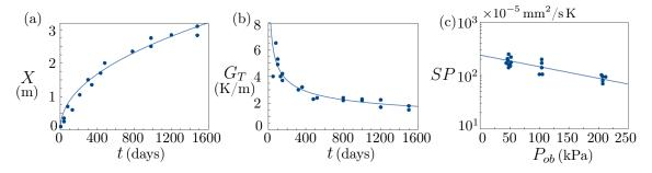
Figure 6: (a) Position of the  $0 \,^{\circ}$ C isotherm X(t) in soil below a buried natural gas pipeline cooled to -8.5  $^{\circ}$ C [64]. (b) Temperature gradient measurements at the position of the freezing front X(t) [64]. (c) Segregation potential data for Calgary silt obtained by Carlson and Nixon [20].
