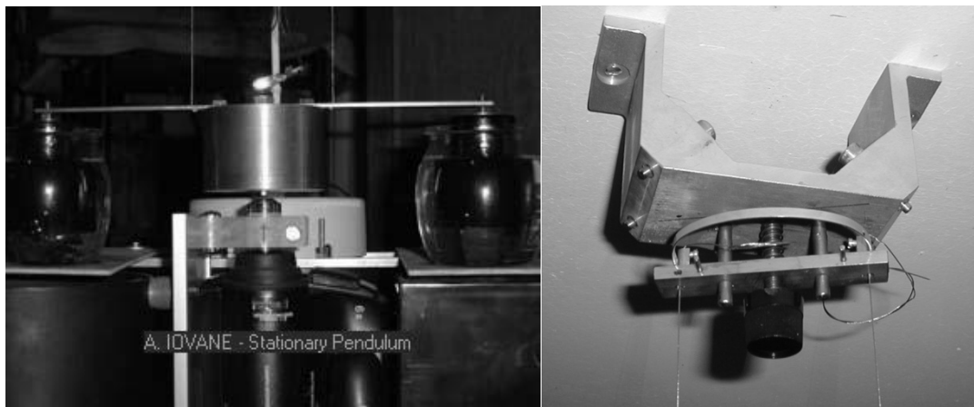
Fig. 1 – Left: the damped bob of the pendulum. Right: the suspension
