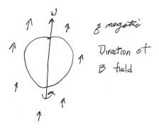
The  $q\mathbf{v}\times\mathbf{B}$  force provides the centripetal force necessary to keep the electron, quark or proton at constant radius instead of bulging at the equator due to centrifugal forces.
