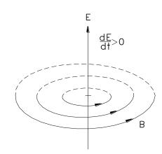
Fig.1 : Direction of the induced magnetic field **B** when  $d\mathbf{E} / dt > 0$  ( **E** increases with time ).
