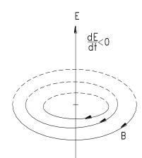
Fig.2 : Direction of the induced magnetic field **B** when  $d\mathbf{E} / dt < 0$  ( **E** decreases with time ).
