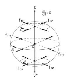
Fig.7 : the magnetic forces **fm** produced on all surface dipoles are radial from centers lying along the axis **OE**.
