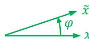
Figure 2: The \tilde{x} -axis as a rotation of the x -axis over a given angle \varphi .
