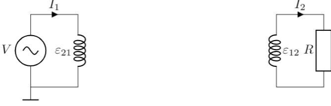
Figure 4. Transformer, the secondary coil is far away from the primary coil, so the retarded effect must be considered.
