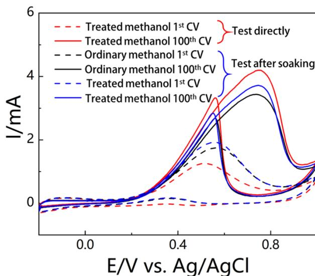
Figure 2. The polarization curve for methanol oxidation before and after electron-attacking treatment for methanol molecules.
