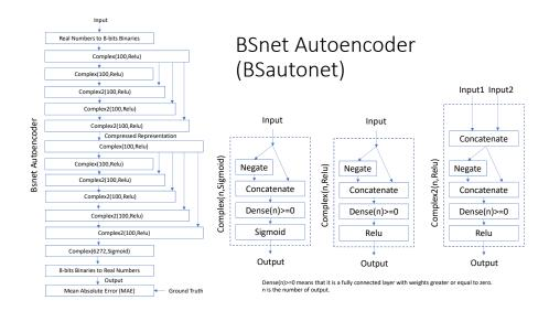
Figure 1: Network Diagram of BSnet Autoencoder (BSautonet))
