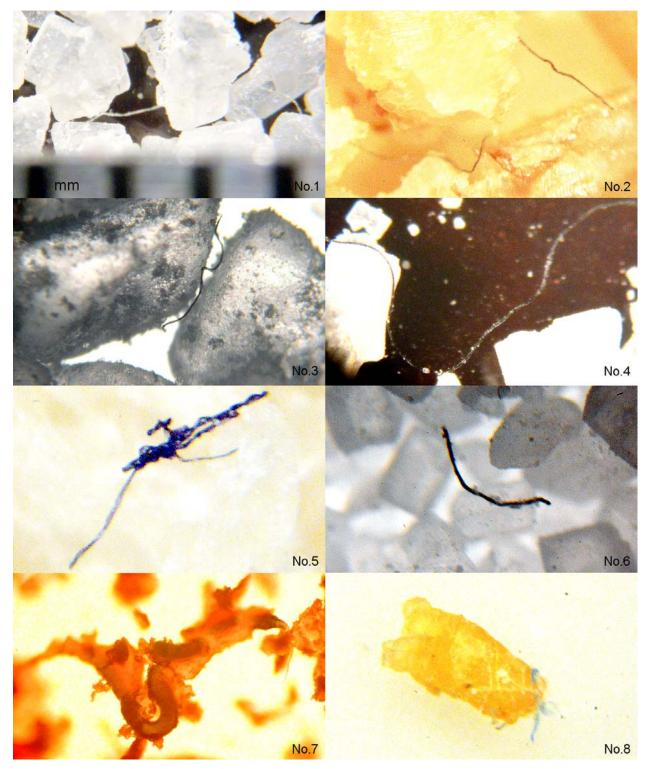
**Micrographs: No.1** Sugar Crystals with Filament, **No.2** Cereal with Filament, **No.3** Sea Salt Crystals with Filament, **No.4** Sugar Crystals with Filament, **No.5** Brioche Baguette with Filament, **No.6** Black Filament in Sugar Crystals, **No.7** Filament imbedded with Liquid, **No.8** Filament wrapped food granule.
