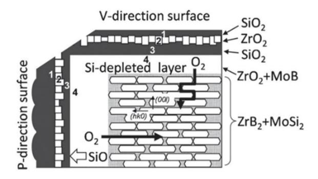
**Fig. 5.** Schematic representation of both V- and P-direction cross sections in textured ZrB<sub>2</sub>–MoSi<sub>2</sub> ceramics oxidized for four h at 1500°C, illustrating anisotropy in oxidation behaviour [56].
