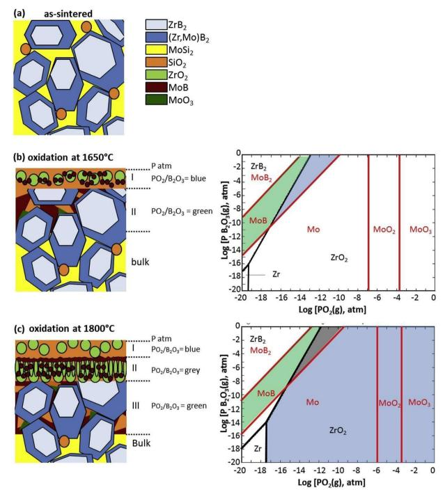
**Fig. 4** Left-hand side: Schematic of microstructural evolution starting from (**a**) as-sintered state up to oxidation at (**b**) 1650 and (**c**) 1800 °C. Right-hand side: phase stability diagrams for the Zr-B-O (black) and Mo-B-O (red) system as a function of partial pressures of oxygen and boron oxide at (**b**) 1650 °C and (**c**) 1850 °C [30].
