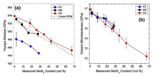
**Fig. 6 (a)** Young's modulus and **(b)** Vickers microhardness as a function of MoSi<sub>2</sub> content in ZrB<sub>2</sub>-MoSi<sub>2</sub> ceramics. N, M and C indicate coarse, medium and fine powder grades of ZrB<sub>2</sub>, respectively. X indicates vol.% of MoSi<sub>2</sub>. In part **(a)**, ROM refers to volumetric rule of mixtures [57].
