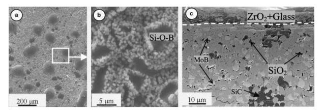
**Fig. 2** SEM images showing (**a, b**) Surface and (**c**) Cross-section of ZrB2 –20 vol.% MoSi<sub>2</sub> oxidised at 1000°C [41].
