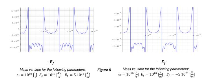
From the period of the mass plot, we determine that the oscillation frequency is approximately:  $f = 1.6 \ 10^{14} \ [Hz]$
