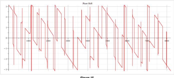
*Figure 15 Phase shift for the following parameters:*  $\omega = 10^{10} \left[\frac{1}{s}\right] E_s = 10^{18} \left[\frac{V}{m}\right] E_f = 5 \ 10^{21} \left[\frac{V}{m}\right]$
