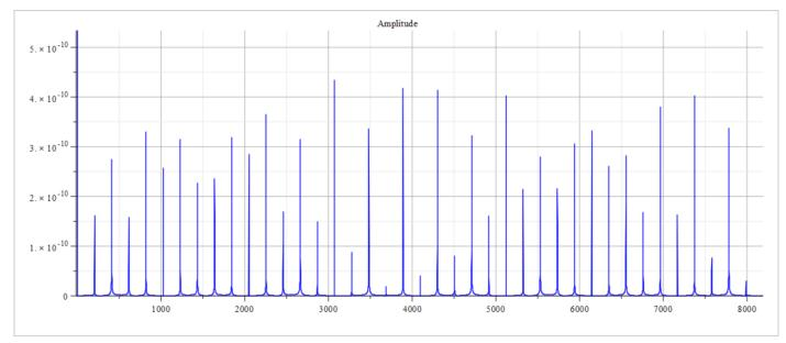
**Figure 16** Frequency spectrum for the following parameters:  $\omega = 10^{10} \left[\frac{1}{s}\right] E_s = 10^{18} \left[\frac{v}{m}\right] E_f = -5 \ 10^{21} \left[\frac{v}{m}\right]$
