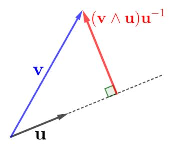
Figure 4: The red vector is the "rejection" of  $\mathbf{v}$  with respect to  $\mathbf{u}$ .
