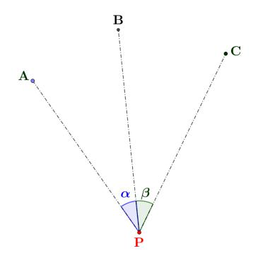
Figure 1: The points A, B, C and the angles  $\alpha$  and  $\beta$  are known. Determine the location of the observer point P.
