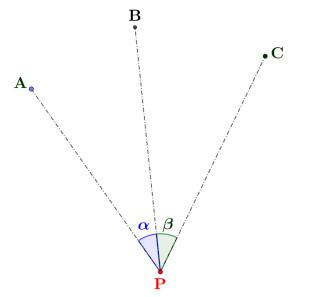
The points A, B, C and the angles  $\alpha$  and  $\beta$  are known. Determine the location of the observer point P.
