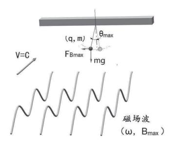
Figure 3.2 Lorentz magnetic field force of a charged stationary ball in a sinusoidal magnetic field wave
