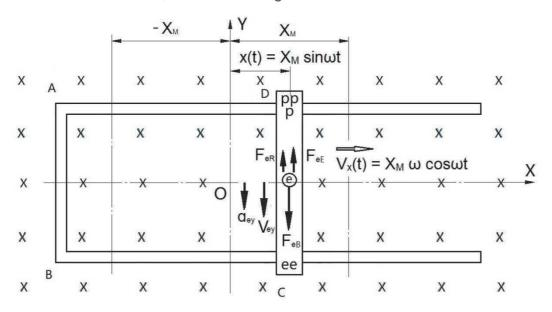
Figure 2.2 Electromotive force of wire CD moving back and forth sinusoidally
