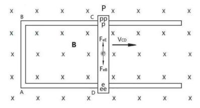
Figure 1.3 Force analysis of electrons in metal wire CD
