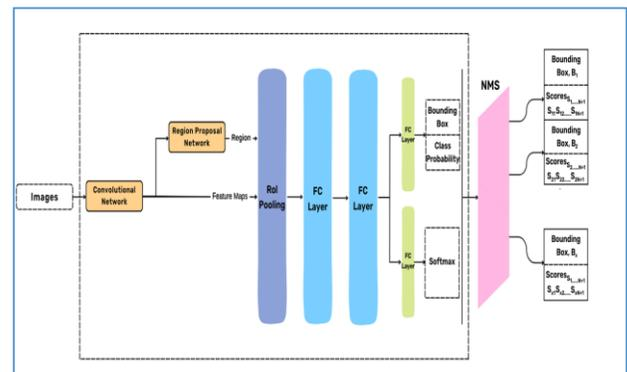
Figure 3: Architecture of Faster RCNN
