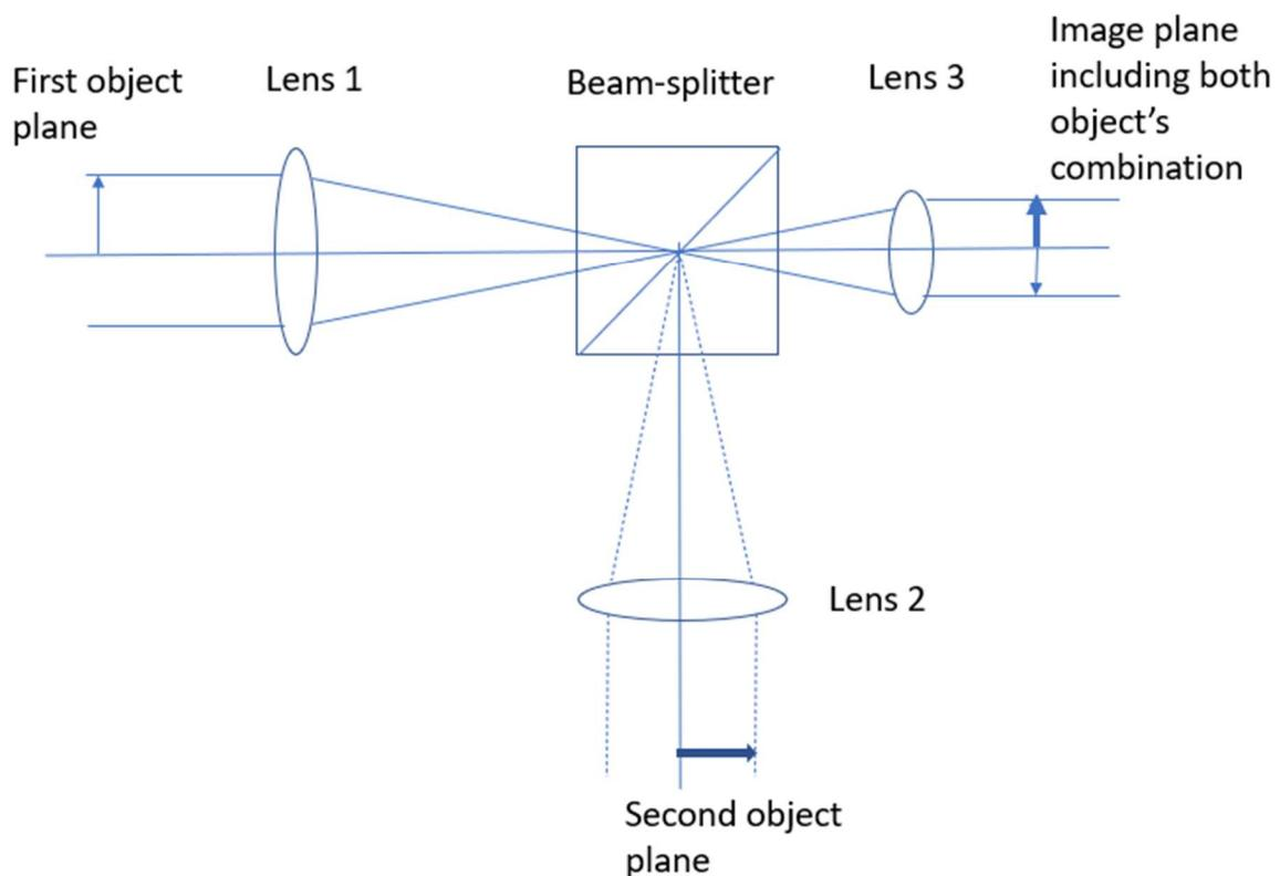
Fig. 2 Optical schematic of the optical system that projects two objects located in different planes into one image plane
