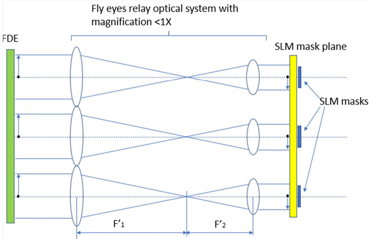
Fig. 1 The Fly-eyes relay optical schematic
