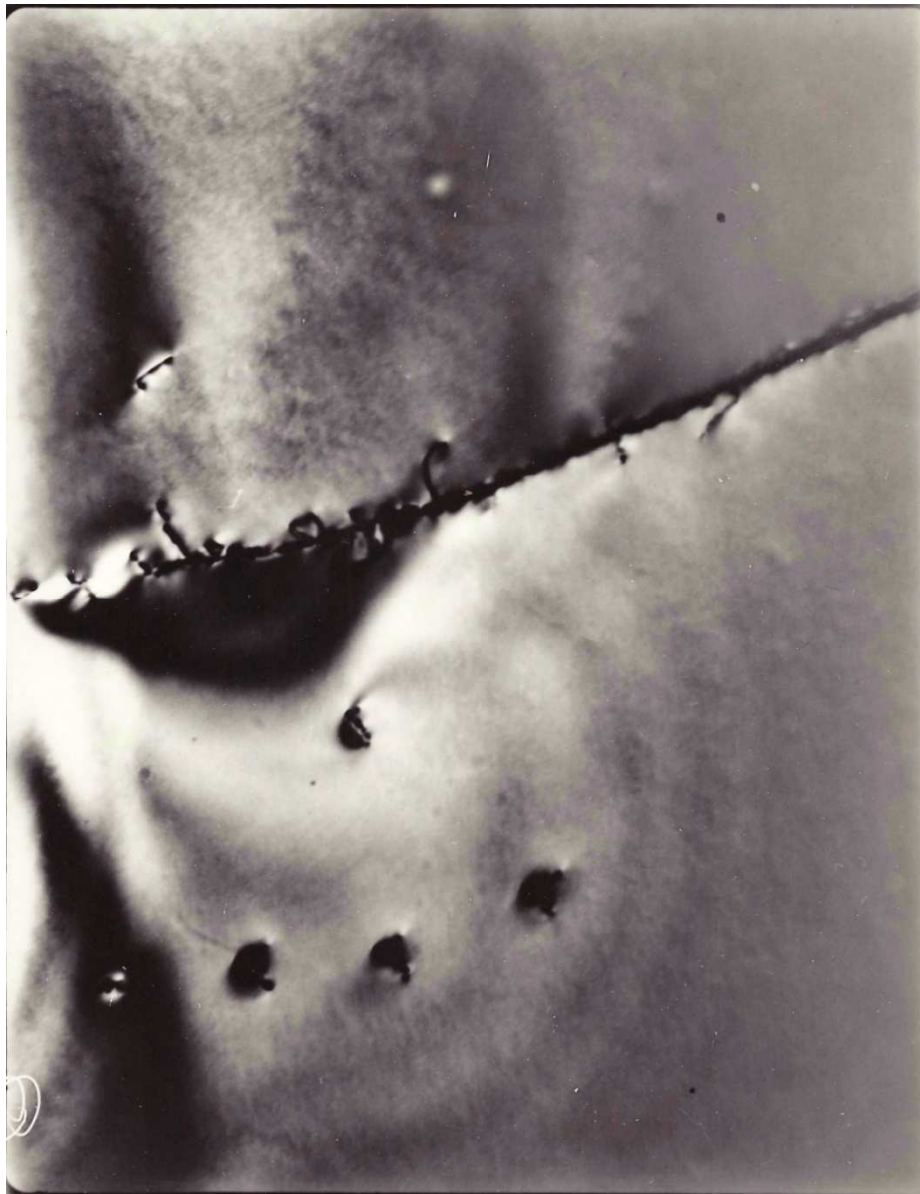
Figure 204. TEM Photo of Gold Ribbon Foil Specimen 3020 following an (900, 340, t_A = 1 hour) Q&A Series Treatment. Note tangled subgrain boundary wall of dislocations and the presence of black spot secondary defects in regions away from various dislocation structures.
