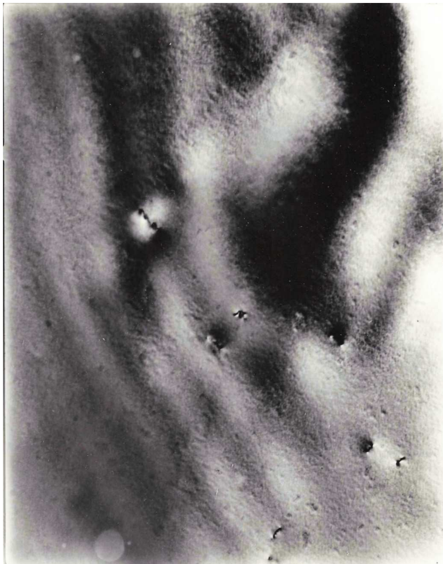
Figure 205. TEM Photo of Gold Ribbon Foil Specimen 3020 following an (900, 340, t_A = 1 hour) Q&A Series Treatment. Calculated dislocation sink density = 2 \times 10^8 \text{ cm}^{-2} .
