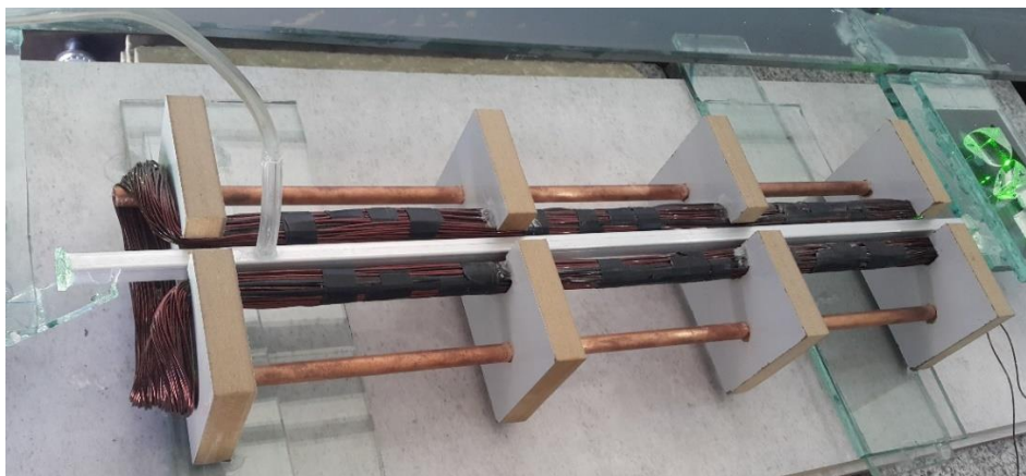
Fig. 8 Longitudinal electrical magnet with two parallel rows of a coiled wire
