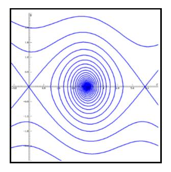
Fig. 7: Dissipative pendulum and the formation of a point attractor [4].
