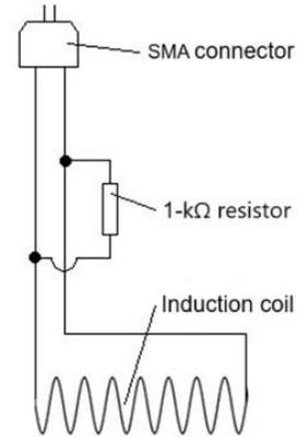
Fig. 2B Schematic of induction coils
