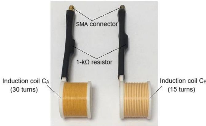
Fig. 2A Photo of induction coils
