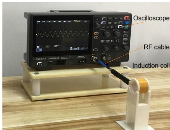
Fig. 3 Photo of oscilloscope with induction coil
