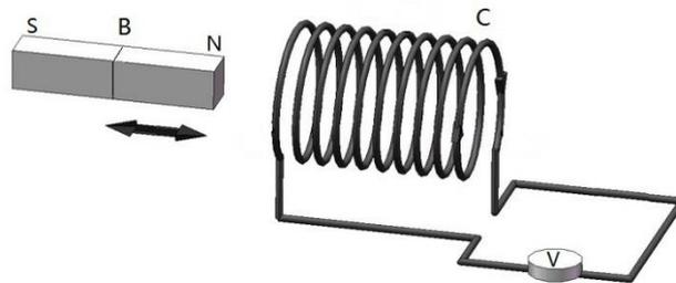
Figure 1 Electromagnetic induction in a metal coil
