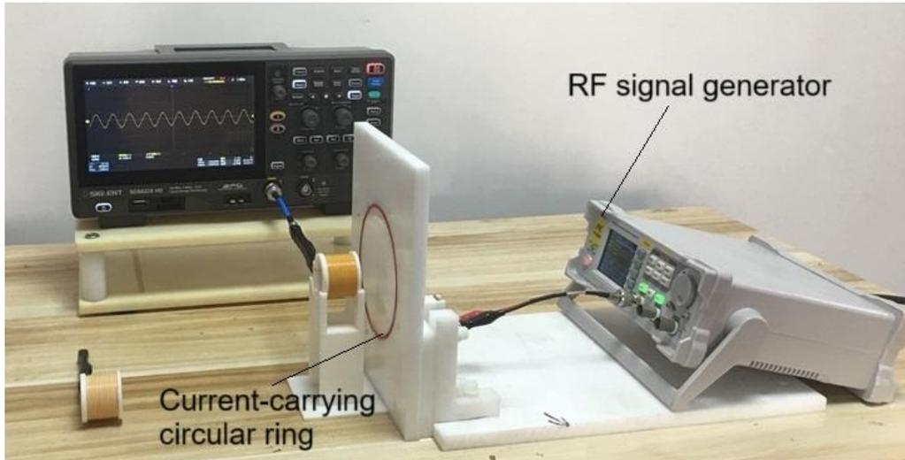
Fig. 5 Induction voltage of coil under RF signals
