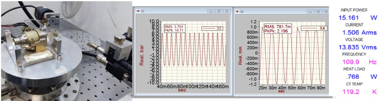
Figure 6: Test bench of the K527-K590 hybrid cryocooler. testing the cold head maximal capacity with full stroke of the cold head and unmatched compressor parameters.
