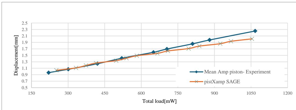
Figure 4: Piston amplitude vs. Total load SAGE Validation
