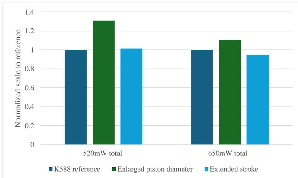
Figure 8: Normalized AC power input at 78C@120K.
