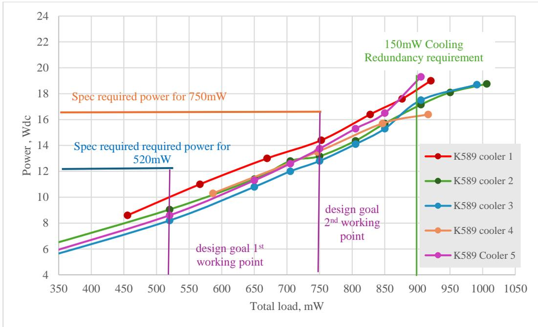
Figure 15: Prototype load line @120K@78°C ambient. The working points are marked to demonstrate the coolers' performance. The data are drawn from the controller input power measurements.
