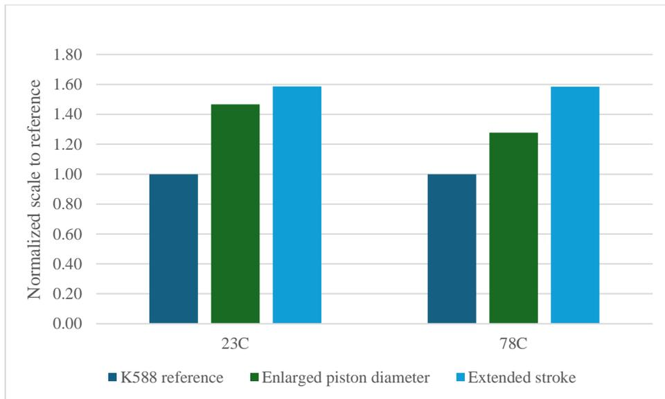
Figure 7: Normalized cooling capacity at 120K.
