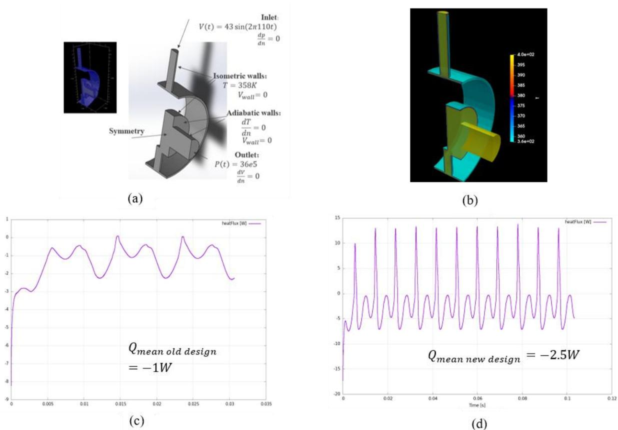
Figure 12: CFD analysis for transient heat transfer from the gas to the solid interface in the cold head ambient rejector.
