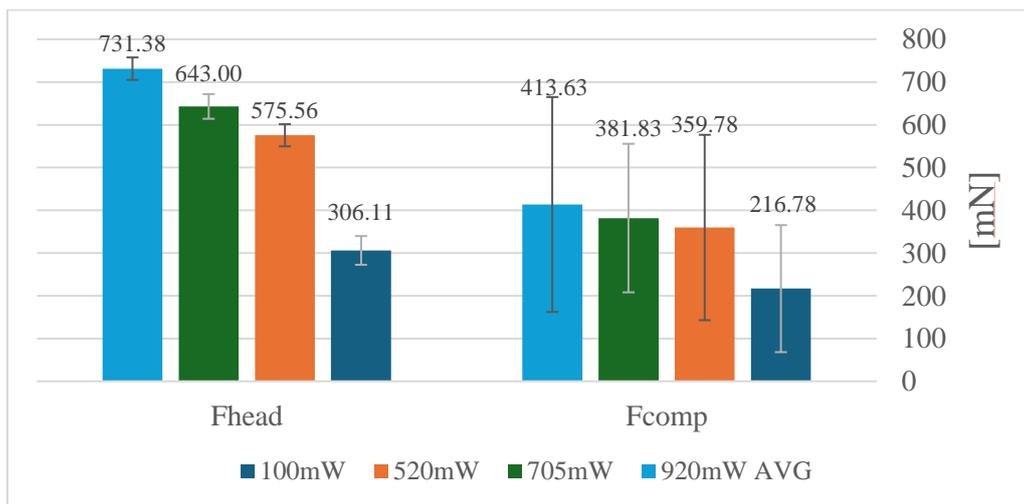
Figure 16: Averaged induced forces measured on 8 prototypes in four different working points. The chart shows the cold heat and compressor stand-alone forces in a 90 degrees setup configuration to eliminate constructive or destructive interferences.
