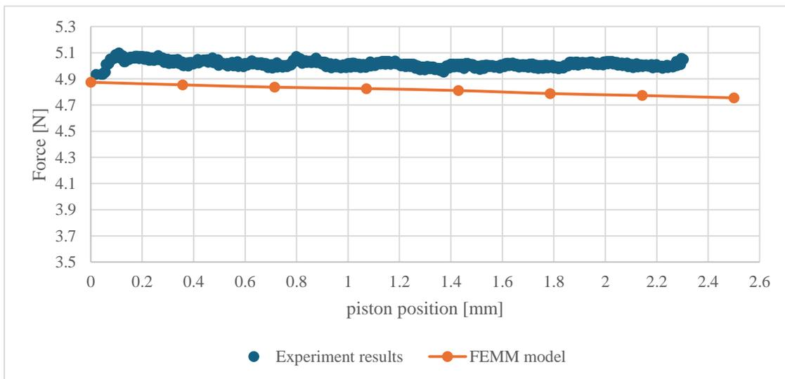
Figure 11: Motor constant validation by experiment vs. FEMM 2D model.
