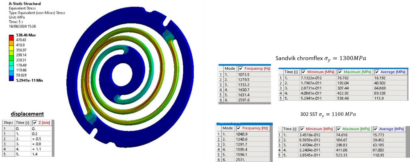
Figure 10: Flexure bearing stress analysis in static displacement conditions.
