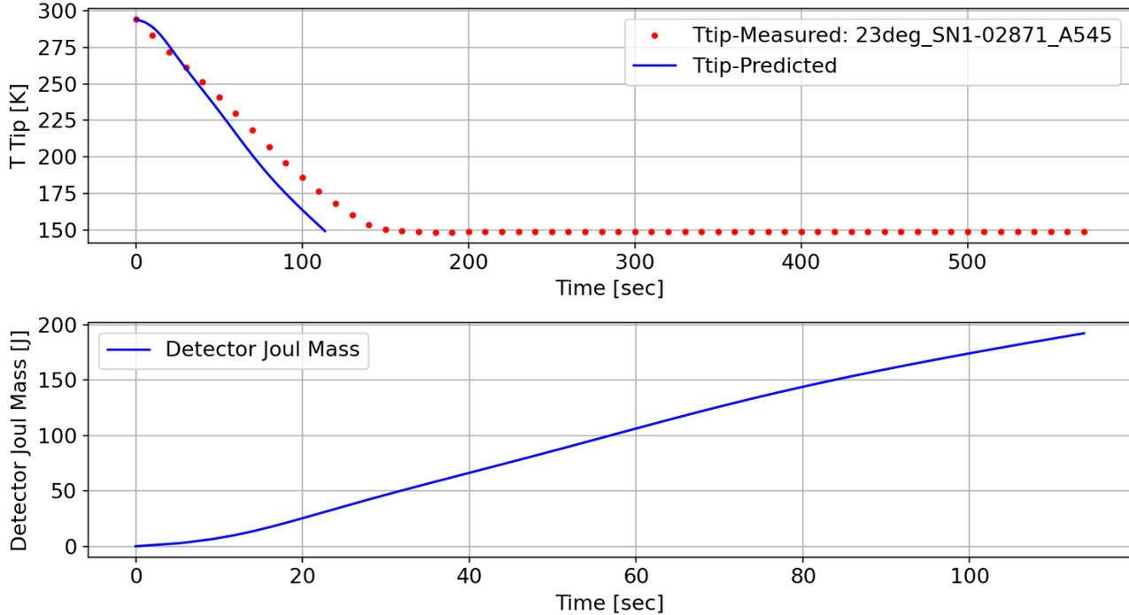
Figure 19: cool-down time tool validation process with the K590 cryocooler CDD data at 23°C. Error value achieved is less than 30% of the experimental values.
