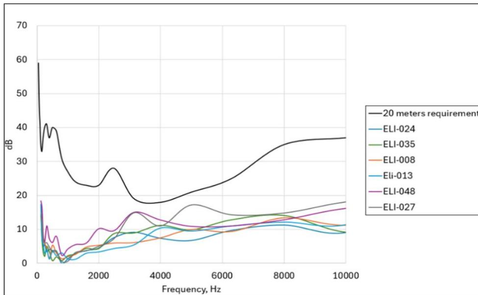
Figure 18: Acoustic noise test: Acoustic noise measured in an anechoic room, hanging on a flexible mount.
