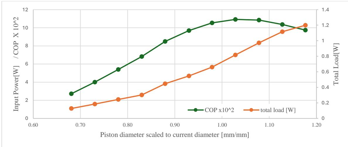
Figure 5: SAGE simulation- Piston diameter effect on performance and cooling capacity.
