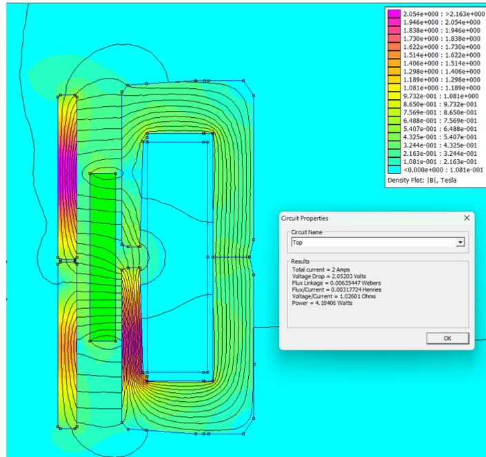
Figure 3: FEMM graphic output of flux intensity field in 2D axisymmetric DC problem.
