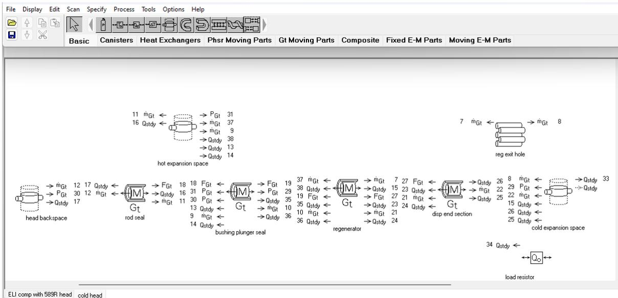
Figure 2: The second level editing window of SAGE® with a model of a cryocooler cold head.
