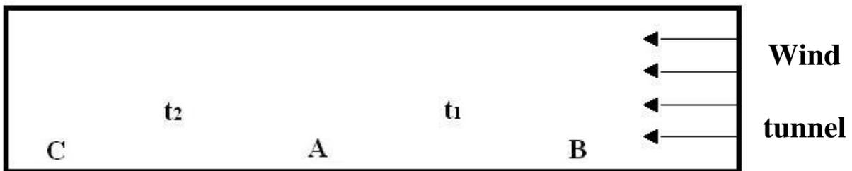
Figure 6. Experimental Setup of the Wind Tunnel Light Speed Test ----Light is emitted from the central point A toward points B and C. Wind flows from right to left. The travel times to B ( $t_1$ ) and C ( $t_2$ ) are compared to test whether light propagation is affected by the moving medium.
